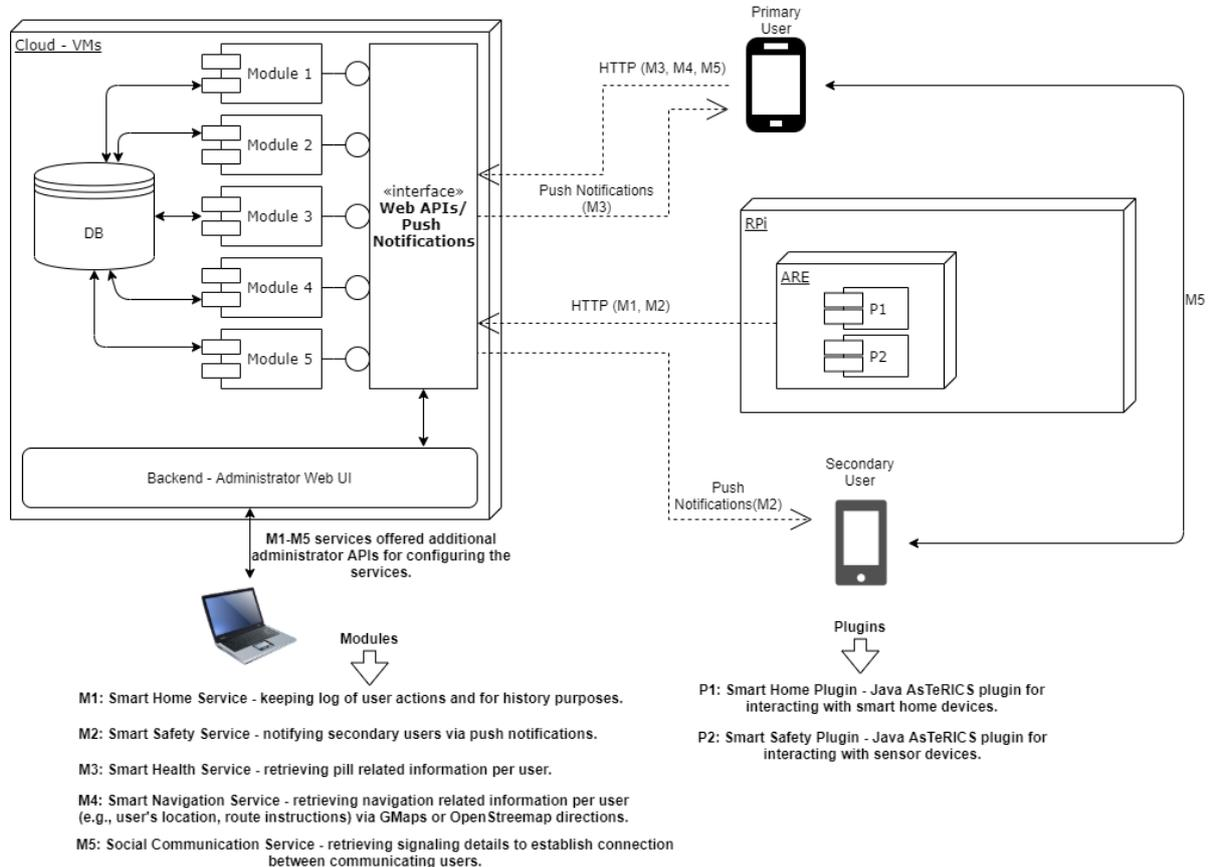
Figure 3: GUIDed high-level architecture
